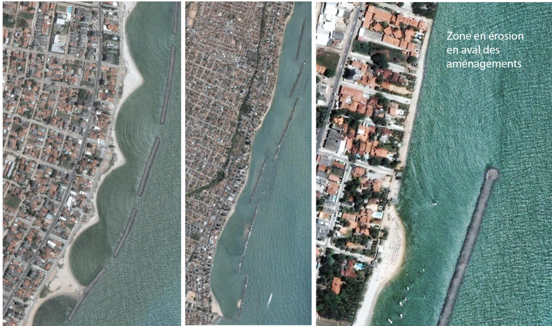
Development of breakwaters in the North East of the Brazil (in the Recife region). From left to right: 1 - former developments, and placing of tombolos; 2 - more recent developments, the effects are not yet very visible; 3 - the beach located downdrift of the developments is being depleted.
