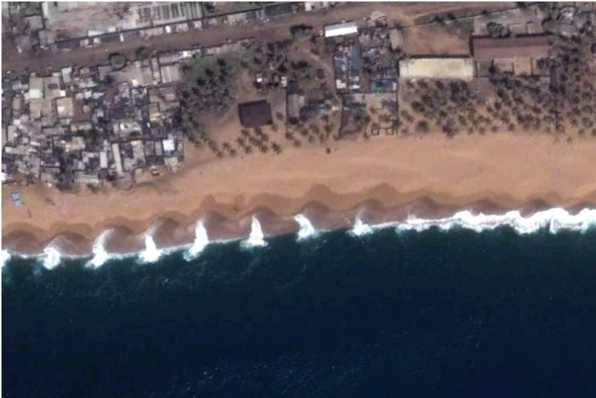
Bar system (ebbing tide - West of the port of Abidjan COTE d'IVOIRE, source: Google Earth)
